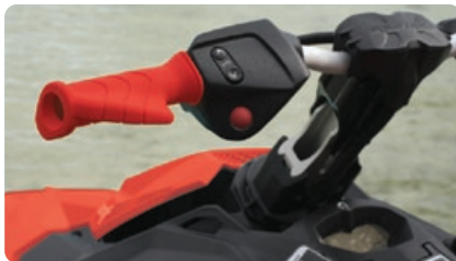
Extended Range VTS™ (Variable Trim System) Offers double the range of the regular VTS™ for greater ease when executing tricks.
