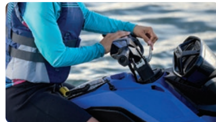
Handlebar With Adjustable Riser A telescopic steering system that optimizes the experience for varying rider sizes.
